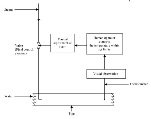
Fig. 11.1 A simple example of manual control; from [3].
