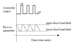
Fig. 11.2 Action of an on/off controller with dead bands; from [6].
