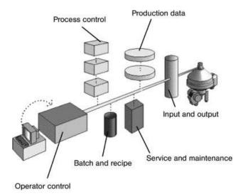
**Fig. 11.7** A typical control system for dairy plant: FOOCOS system from ABB Automation [14]; reproduced with permission.
